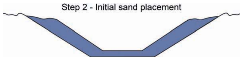
Figure 69.—Initial filter placement.
