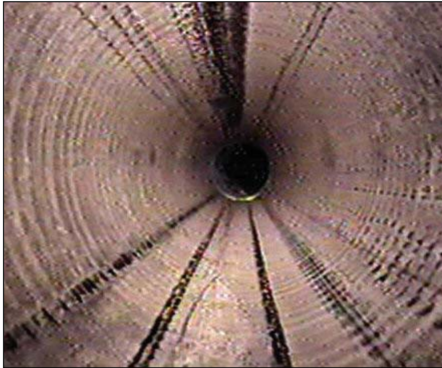
Figure 91. —Profile wall corrugated HDPE pipe has corrugated exterior and smooth interior surfaces.
