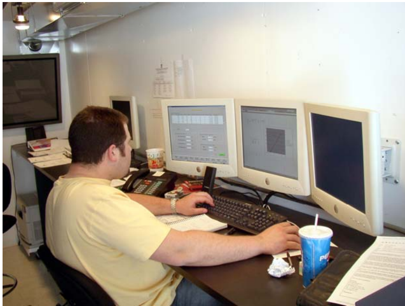
Grouting can now be controlled remotely, by computer, and results evaluated in real time
