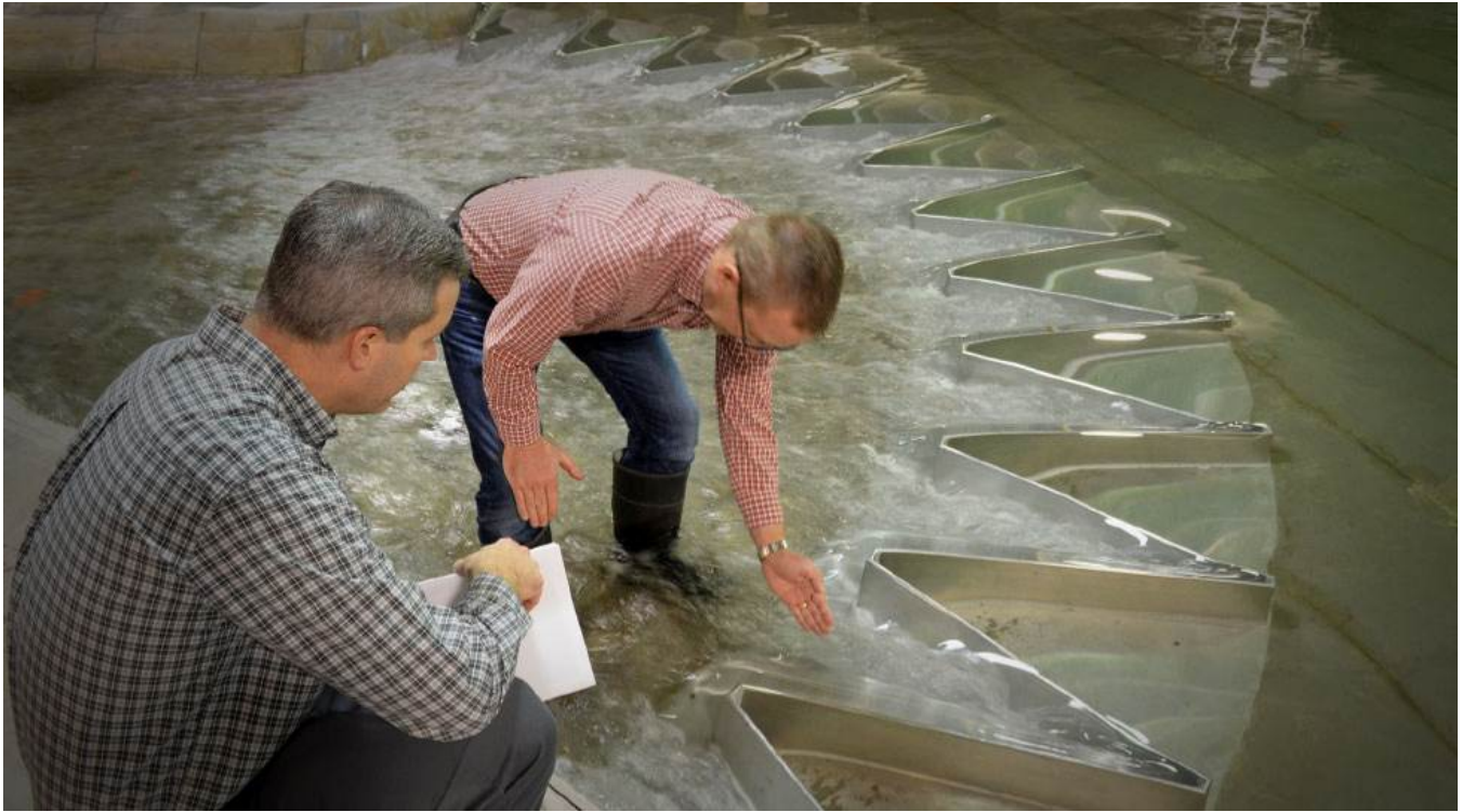
Figure 1. 1:45 scale physical model of the Lake Isabella arced labyrinth spillway at the Utah Water Research Lab (Photo by John Prettyman, U.S. Army Corps of Engineers)
