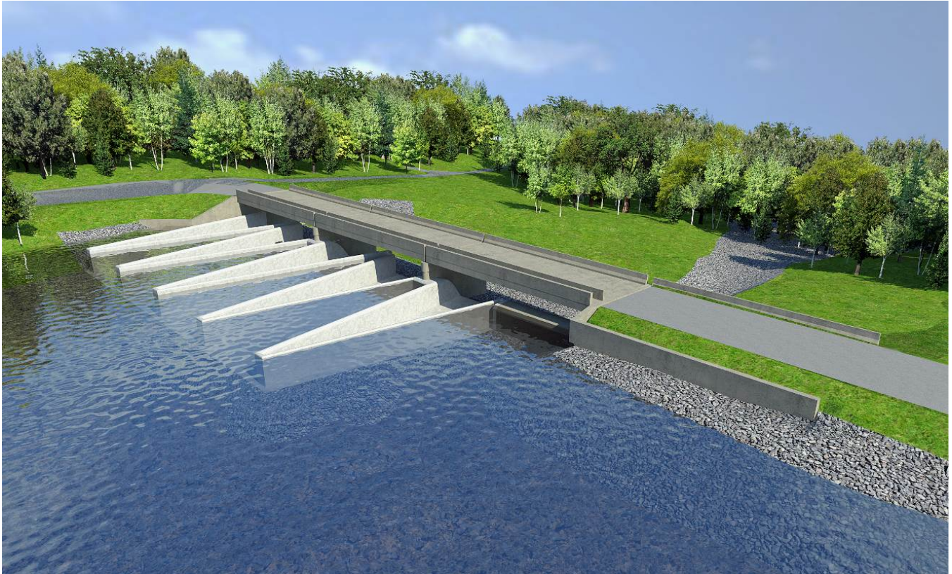
Figure 7. Rendering of proposed labyrinth/ogee spillway at Lake Scranton Dam.
