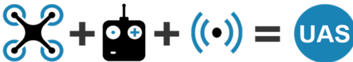
Figure 1: Components of an Unmanned Aircraft System 4
