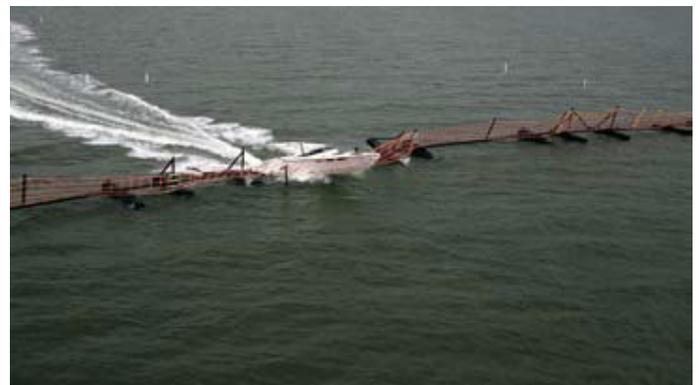
Figure 3: Net Boat Barrier
