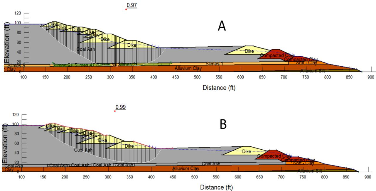
Figure 7. A) Cross section of failed slope in Dredge Cell 2, B) Generalized Section
