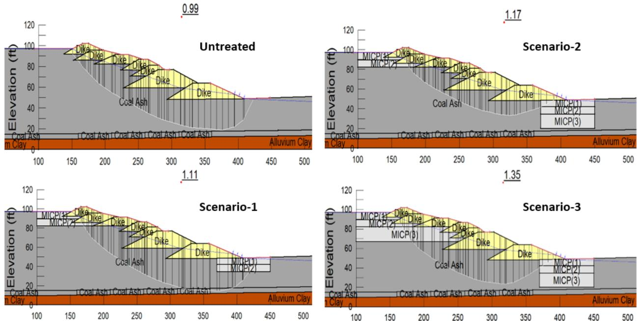
Figure 8. Effect of depth of MICP improved layer on critical failure surface and factor of safety.
