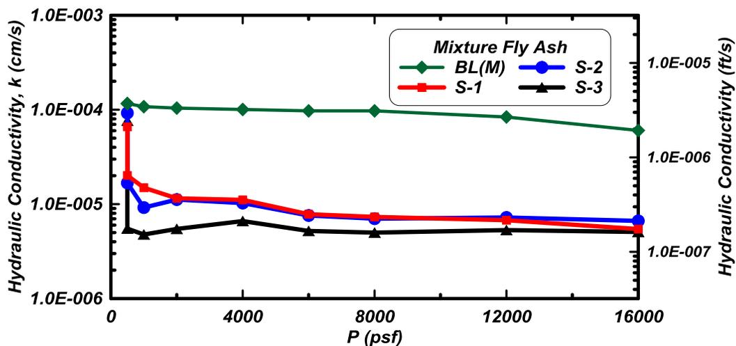
Figure 6. Hydraulic conductivity, modified consolidation test.
