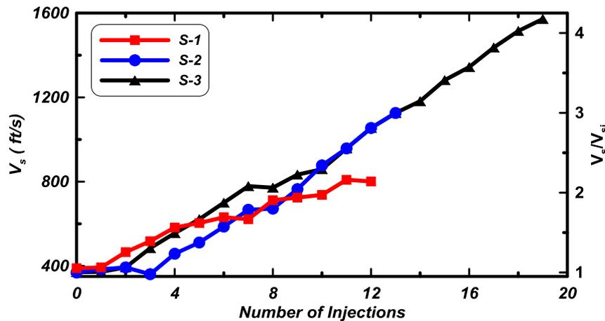
Figure 3. Shear wave velocity during treatment before consolidation test.
