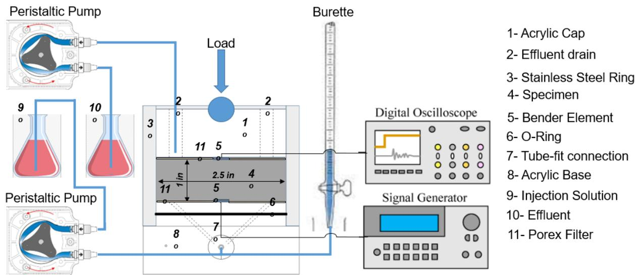
Figure 2. Schematic of devices are used in modified consolidation set-up
