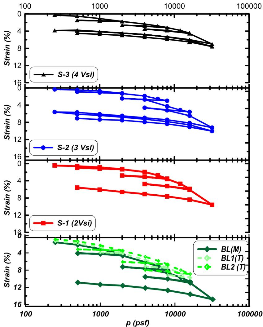
Figure 4. Resultant strain of incremental loading test.
