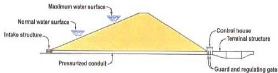
Arrangement 4—Downstream control.—The control feature is located at the downstream end of the conduit.
