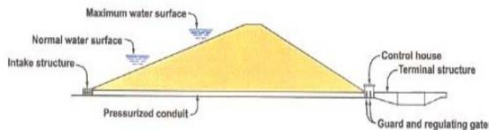
Arrangement 4—Downstream control.—The control feature is located at the downstream end of the conduit.
