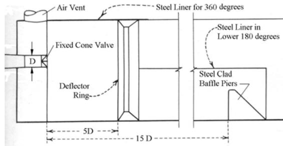
Figure 8. Fixed-cone valve installation
