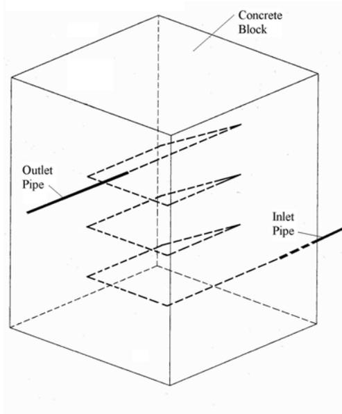
Figure 15. Elbow Energy Dissipator
