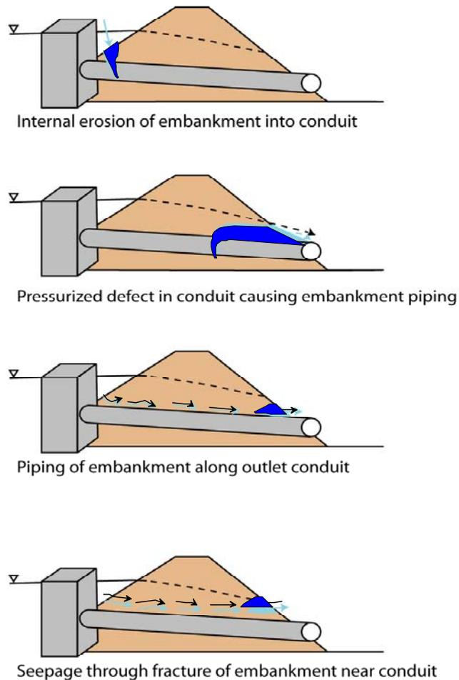
**Figure 1** – Failure Modes for Conduits in Embankment Dams.
