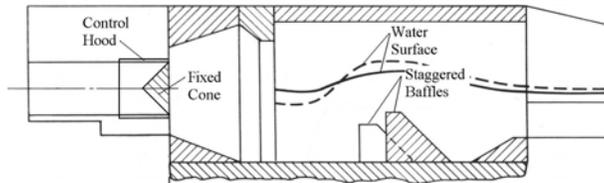
Figure 9. Hooded Installation of a Fixed-cone Valve
