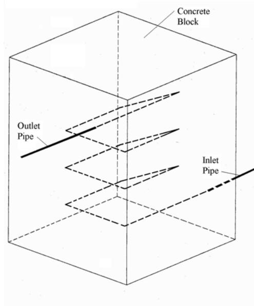
Figure 15. Elbow Energy Dissipator
