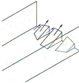
Figure 17. Dentates at the End of Chute
