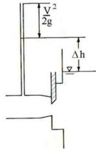
Figure 13. A Sudden Enlargement at the End of a Pipeline
