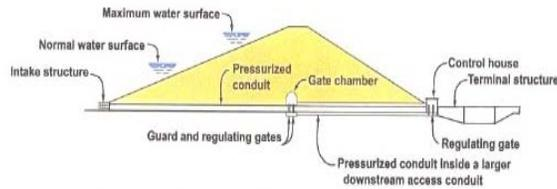
Arrangement 1—Intermediate control with downstream access.—The control feature is located at an intermediate point within the conduit.
