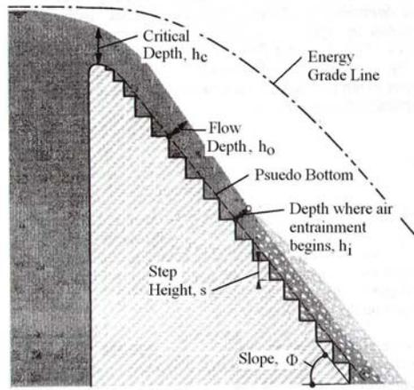
Figure 5. Stepped Spillway
