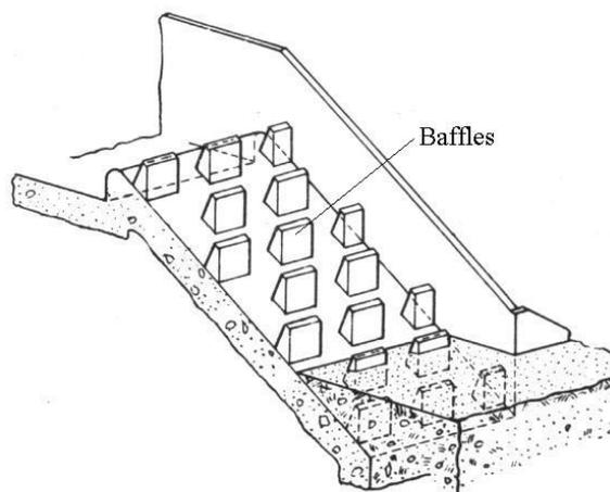
Figure 4. Baffled Apron Drop
