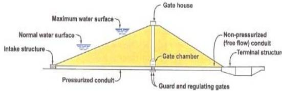
Arrangement 2—Intermediate control without downstream access.—The control feature is located at an intermediate point within the conduit.
