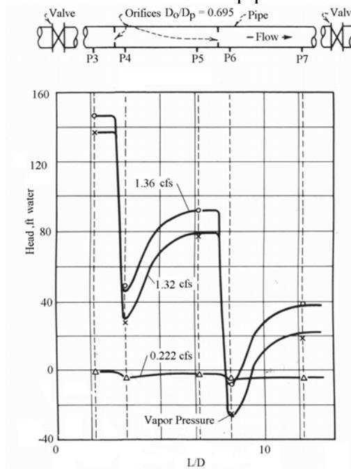
Figure 14. In-line orifices
