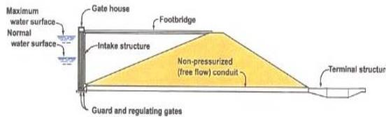
Arrangement 3—Upstream control.—The control feature is located at the upstream end of the conduit.
