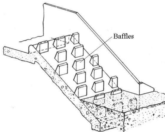
Figure 4. Baffled Apron Drop
