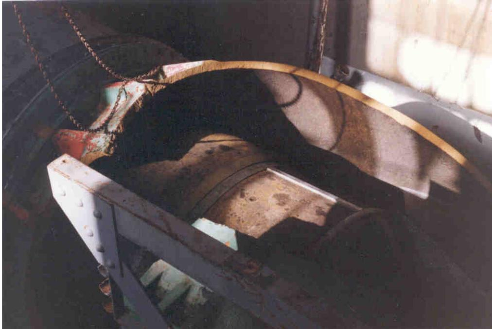
**Photo 4** - Failed needle valve.
