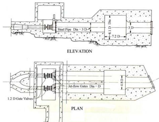
Figure 12. A sudden Enlargement in a Pipeline with Jet Flow Gates
