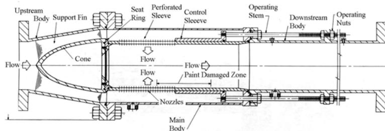
Figure 10. Orifice valve
