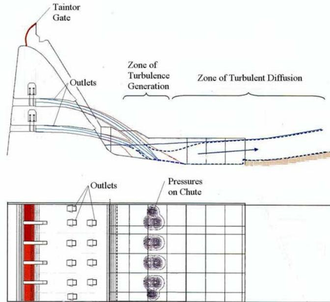
Figure 19. Plunge Pool for an Outlet in a Concrete Dam
