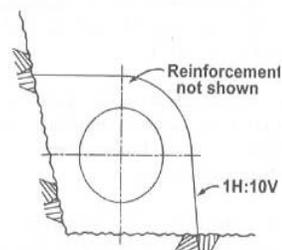
**Figure 2** – Conduit Cast Against Excavated Rock
