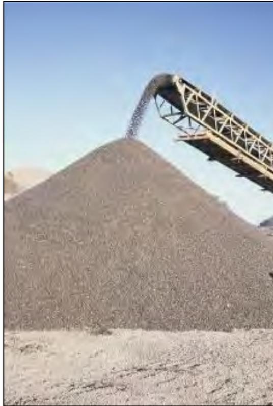
**Figure 7-7. Conical stockpile.**
