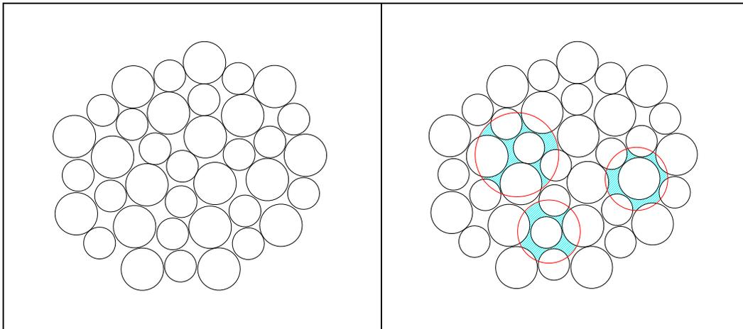
**Figure 6-5. The illustration on the left shows idealized spheres of two sizes and resulting void space between the spheres. For the illustration on the right, three larger spheres (red) are overlain on the original illustration. This demonstrates how the larger spheres will replace once available void space, highlighted in blue.**
