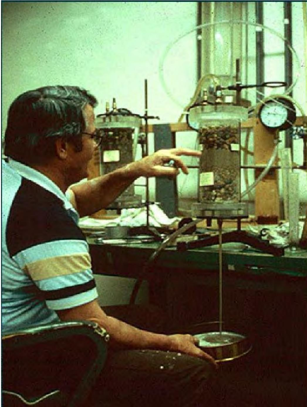
Figure F-3. No erosion filter testing being conducted in Soil Conservation Service laboratory in Lincoln, Nebraska.
