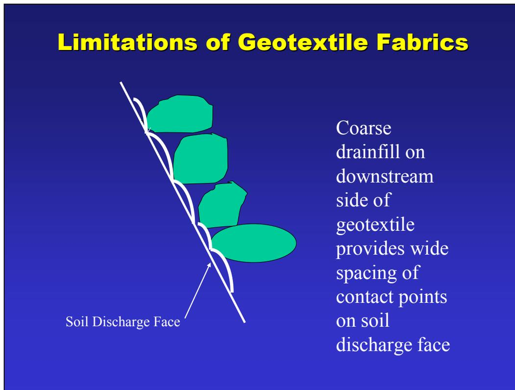
**Figure 3-3. Cross section of a base soil covered by a geotextile that is then covered by coarse gravel. Due to the voids in the gravel, the geotextile can “flex” into these voids, resulting in the loss of positive pressure on the base soil discharge face. Base soil particles can then detach and clog the geotextile.**
