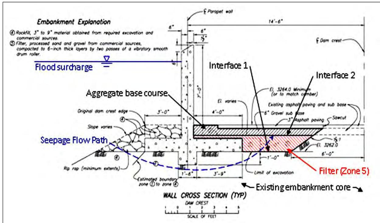
Figure 5-10. Parapet wall cross-section with location of Zone 5 filter and aggregate base course for paving.
