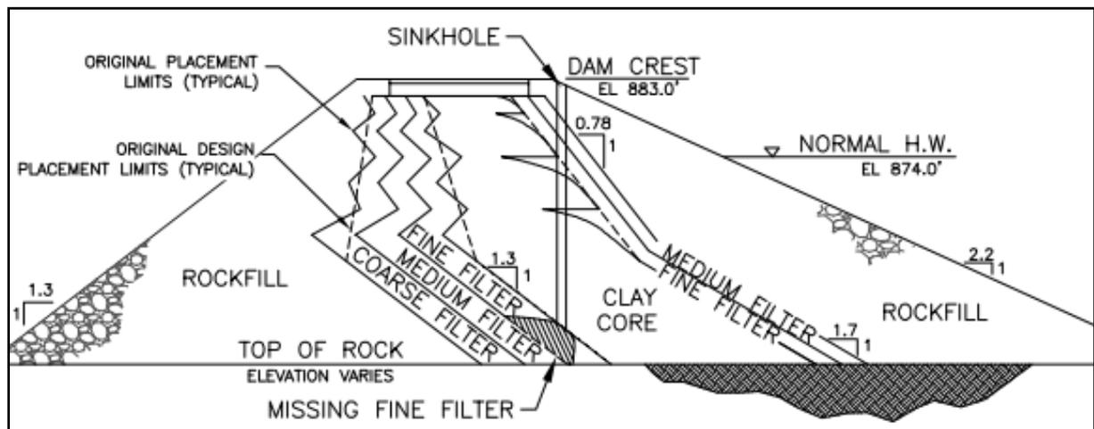
**Figure E-12. Cross section of the original embankment construction showing sinkhole and missing fine filter. Note the “Herringbone” pattern of the downstream filters; original construction placement techniques caused the as-built filter locations (solid line) to deviate from the design placement limits (dashed line).**
