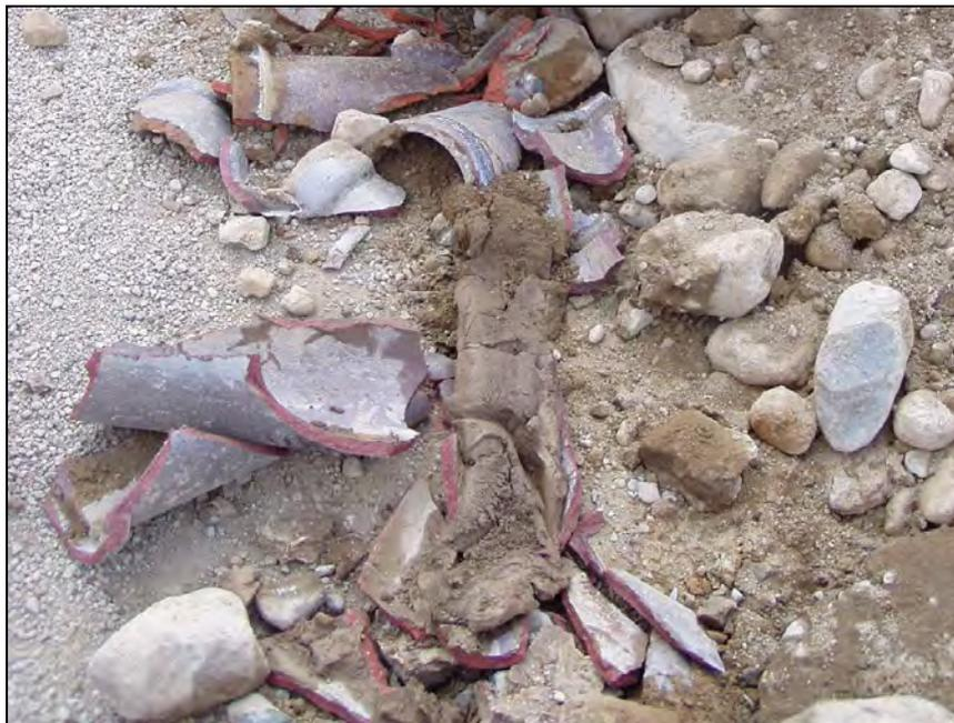
Figure 2-18. Clay tile pipe from 1916 as it was exposed during excavation. Note that the pipe was completely clogged with silt and sand.
