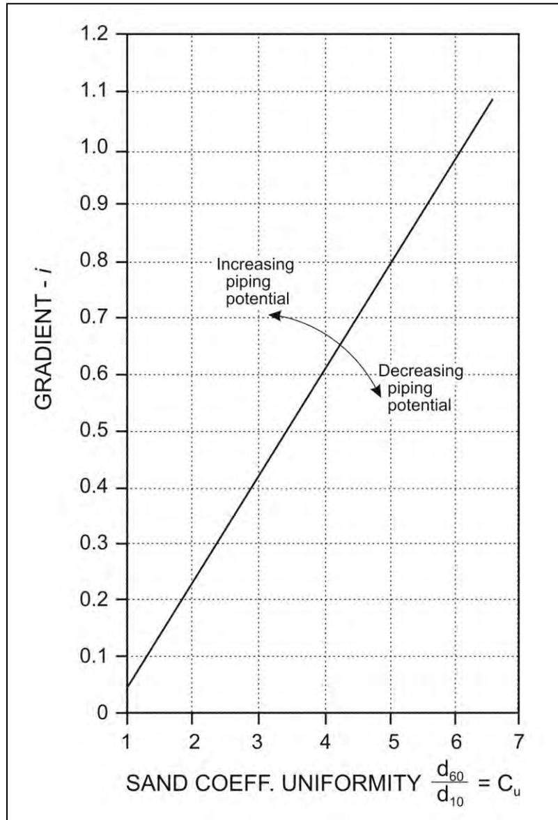
Figure 6-1. Horizontal piping gradient versus coefficient of uniformity.
