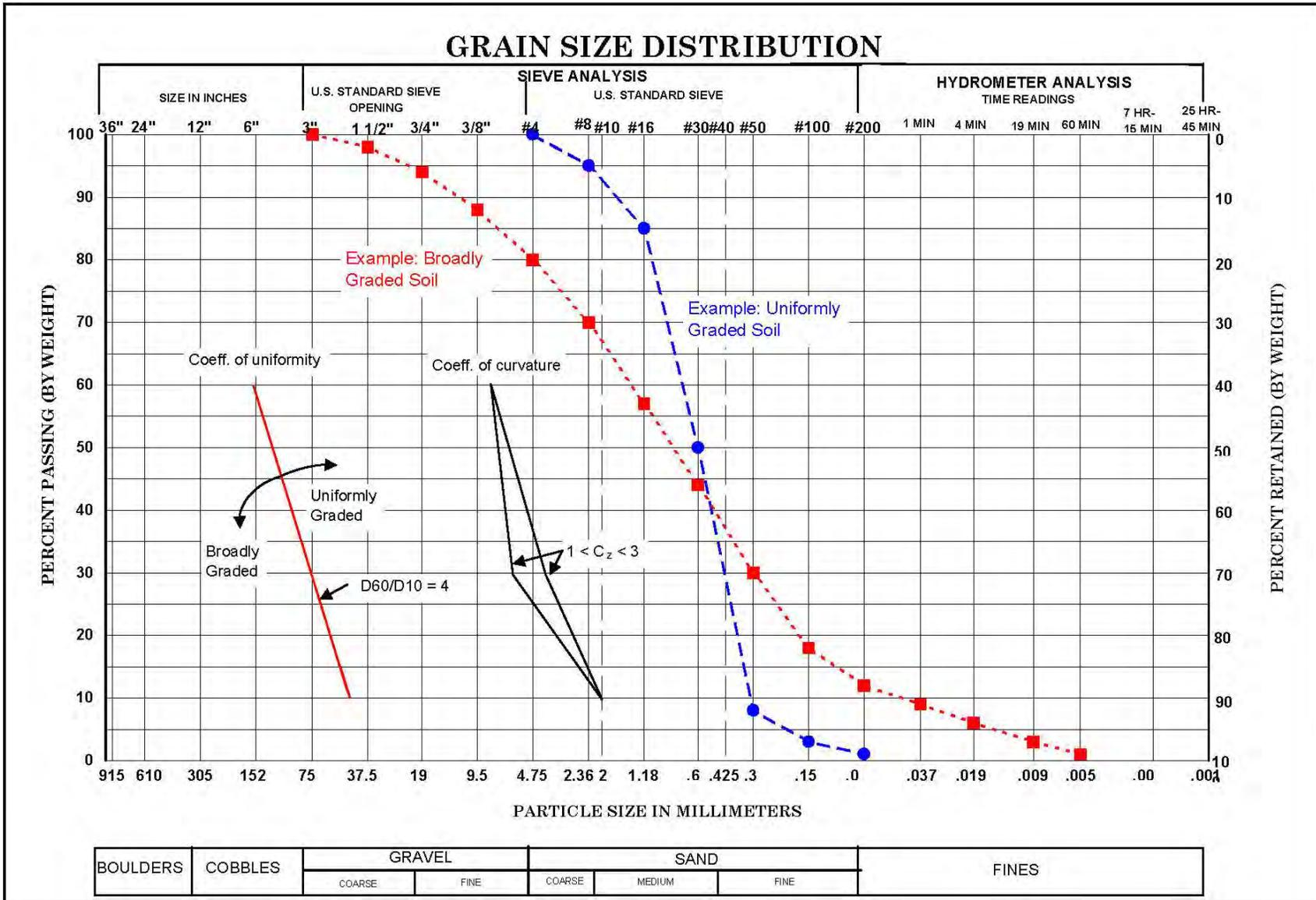
Figure 1. Example of broadly and uniformly graded soils.
