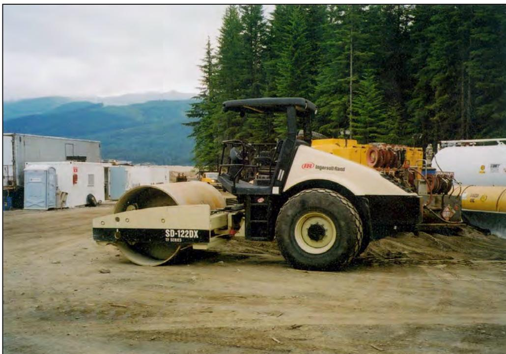
Figure 7-22. Single-drum vibratory roller.
