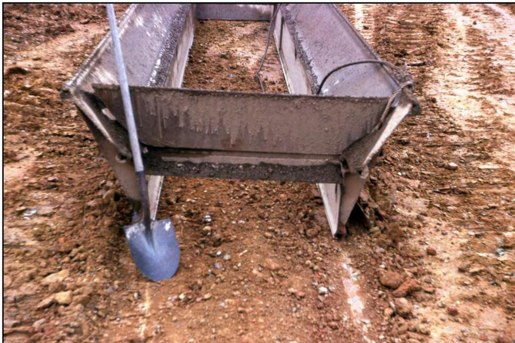
Figure 7-14. Basic single-bin spreader box.
