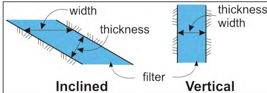
Figure 6-2. Definition of filter width and thickness.
