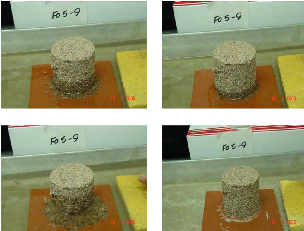
**Figure 4-5. Illustration of relatively poor self-healing behavior. The sample does not collapse well after 50% submersion. The test sequence begins at the lower right photo and progresses counter-clockwise, ending in the lower left photo.**
