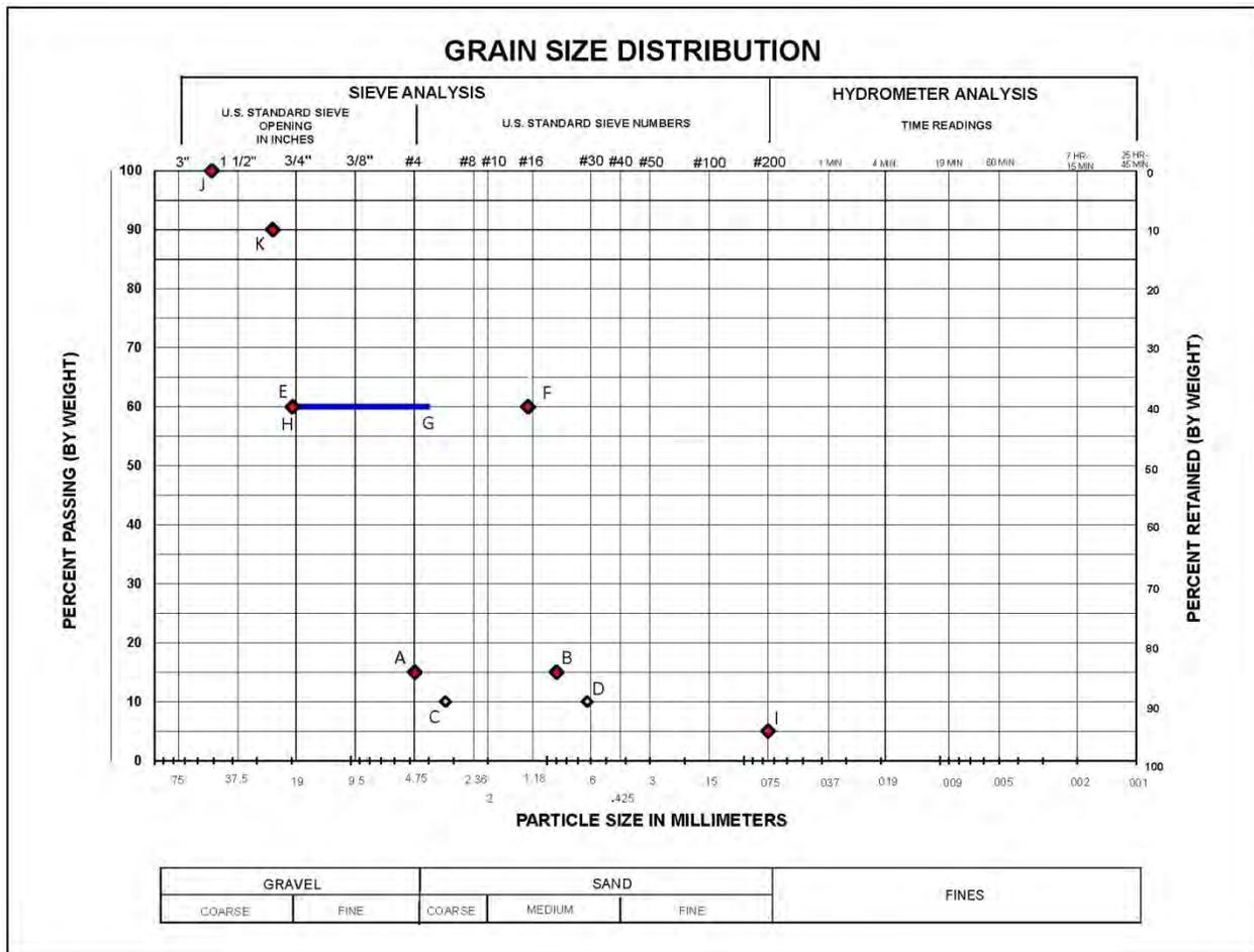
Figure 5-17. Filter Control Points for Interface 2.
