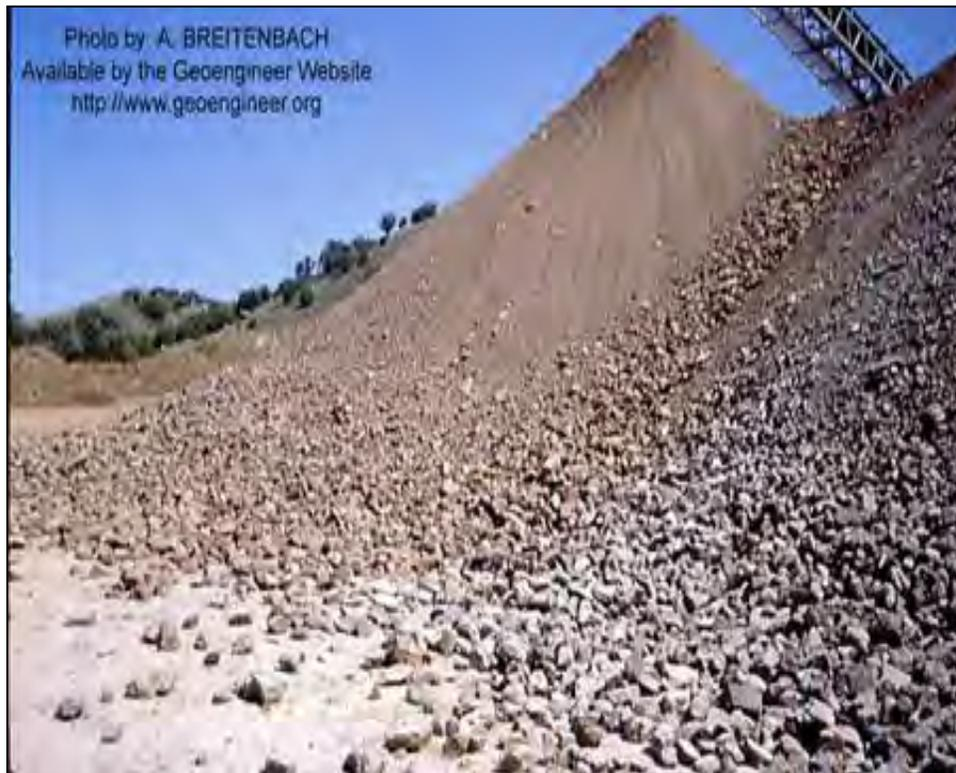
Figure 7-9. Segregation at high cone pile.
