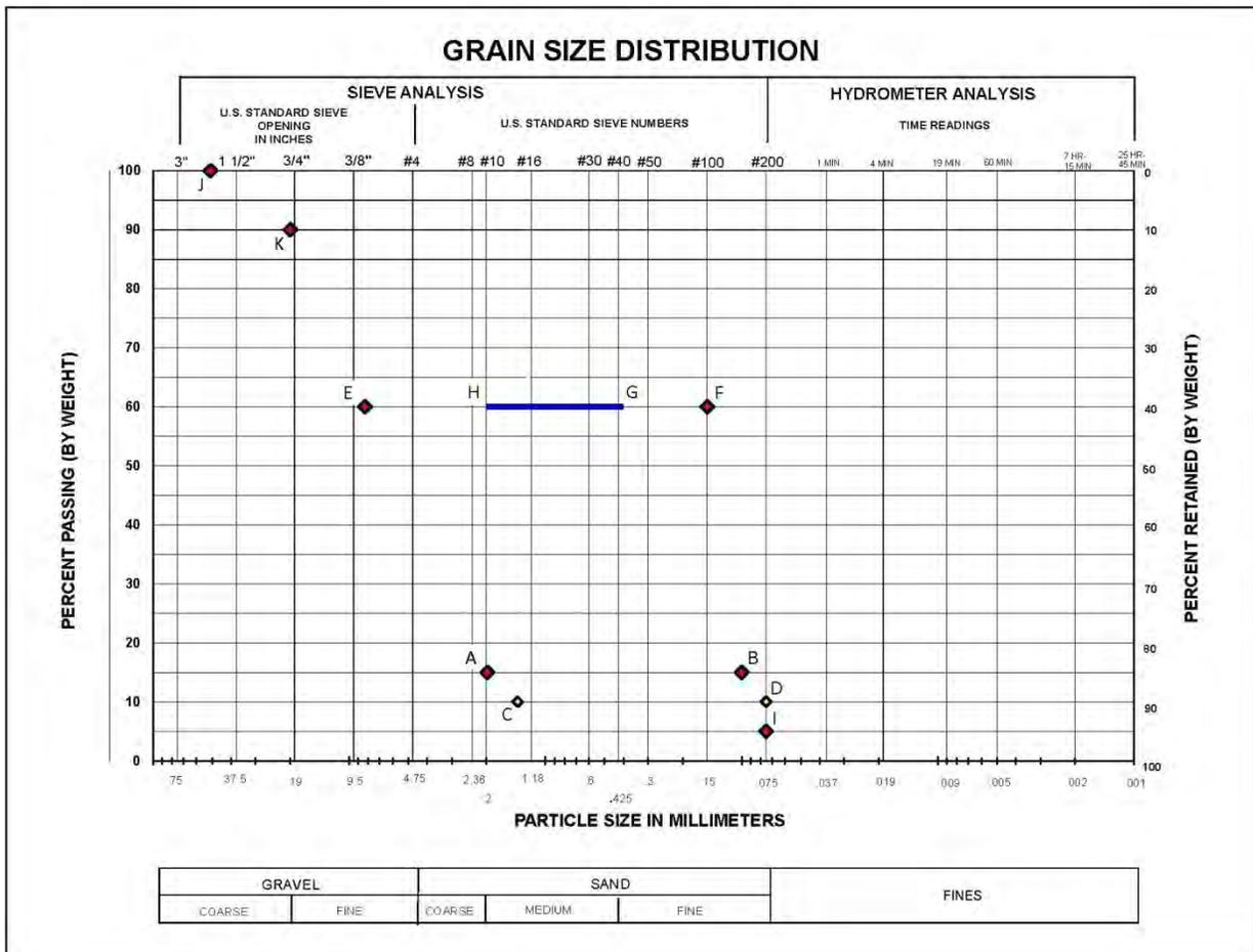
Figure 5-13. Filter control points for Interface 1.
