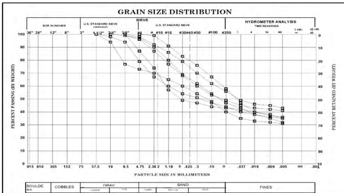
Figure A-1. Gradation plot of example core material.
