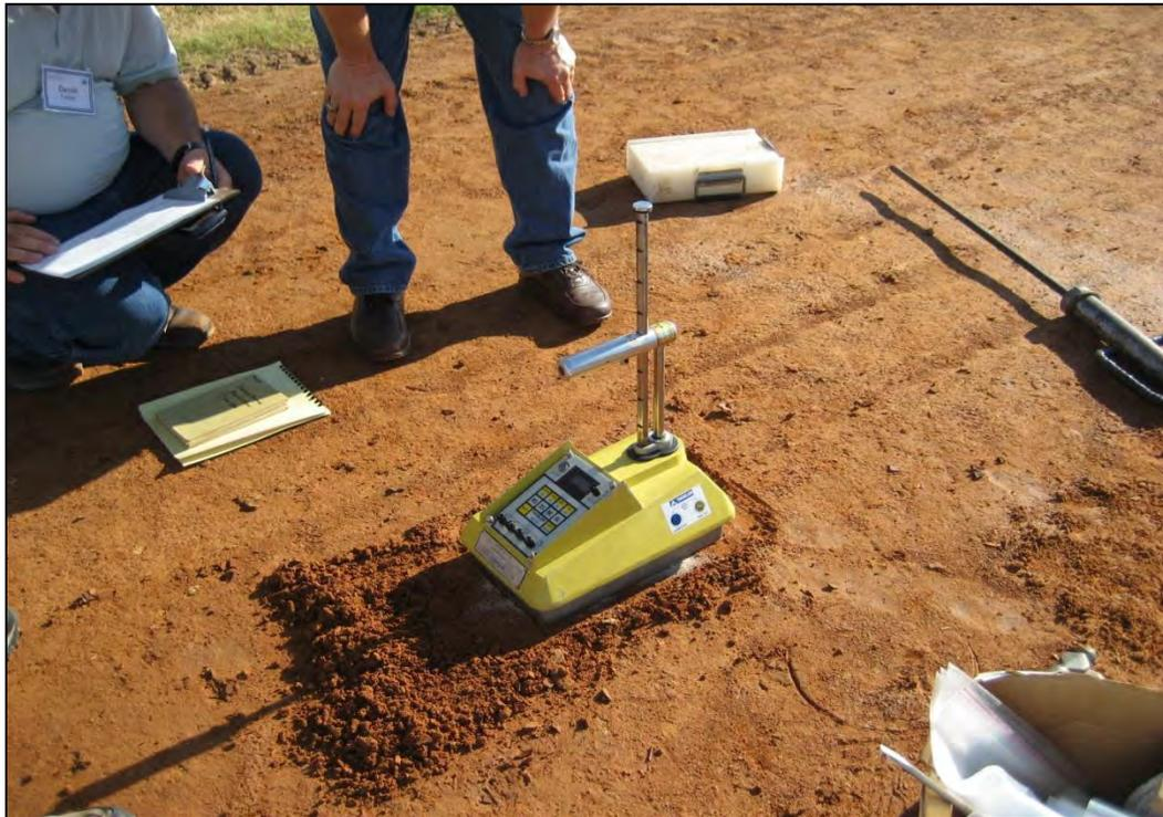
**Figure 7-29. Typical nuclear moisture-density meter.**
