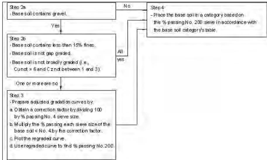
Figure 5-4. Flowchart of the Step 2 process.
