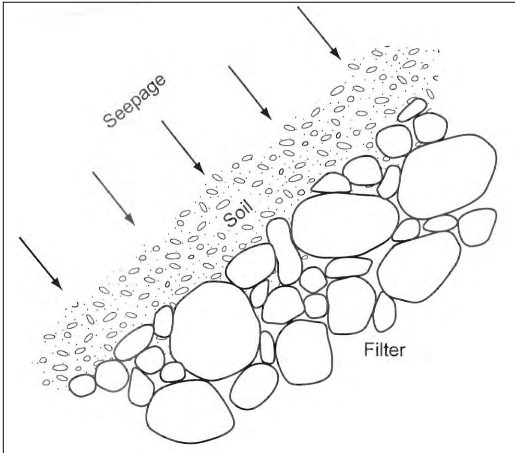
**Figure 1-1. Schematic demonstrating the manner in which a properly designed filter prevents the movement of base soils by seepage forces at the discharge face. The filter supports the discharge face with closely spaced contact points as compaction melds the two zones together such that bridging between the contact points prevents any movement of base soil particles into the filter. At the same time, the filter is sufficiently coarse to allow seepage water to escape freely.**
