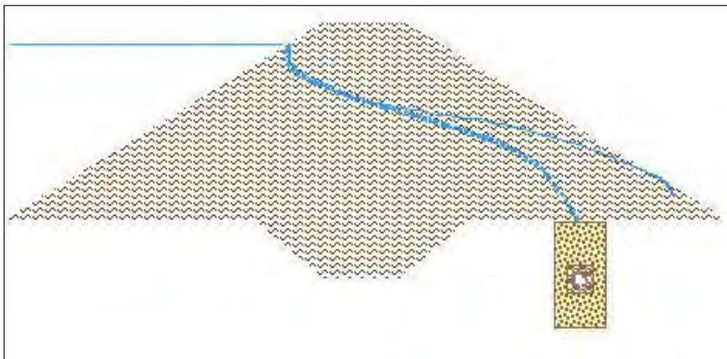
**Figure L-31-1. Foundation trench drain placed inside the downstream embankment section in an attempt to both collect foundation seepage and lower the phreatic line. In anisotropic embankments, this dual function is not likely to be successful.**
