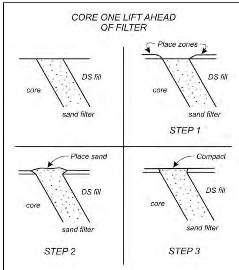
**Figure 7-1. Steps in maintaining impervious core one lift ahead of a chimney.**
