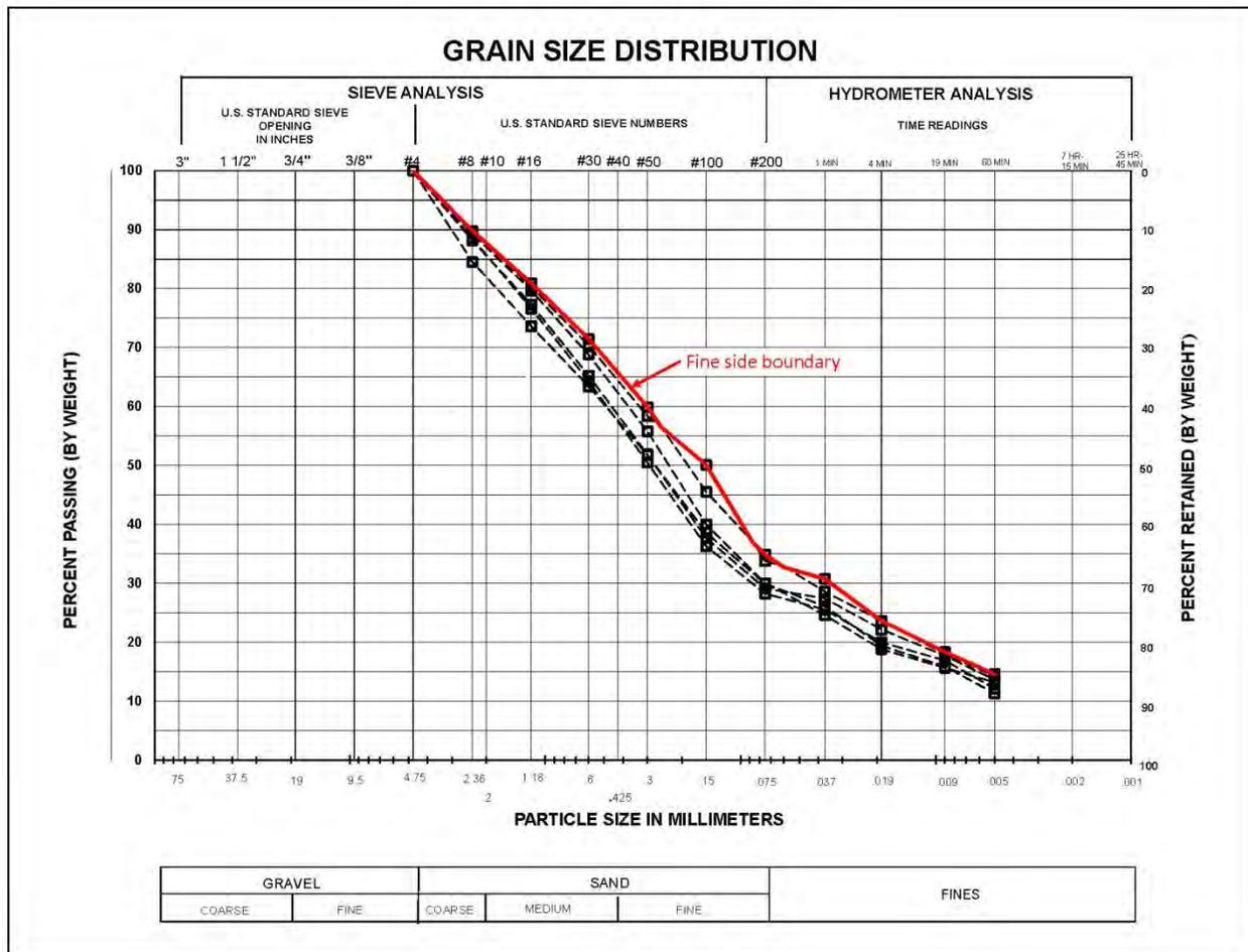
Figure 5-12. Existing embankment dam core gradations after re-grading.
