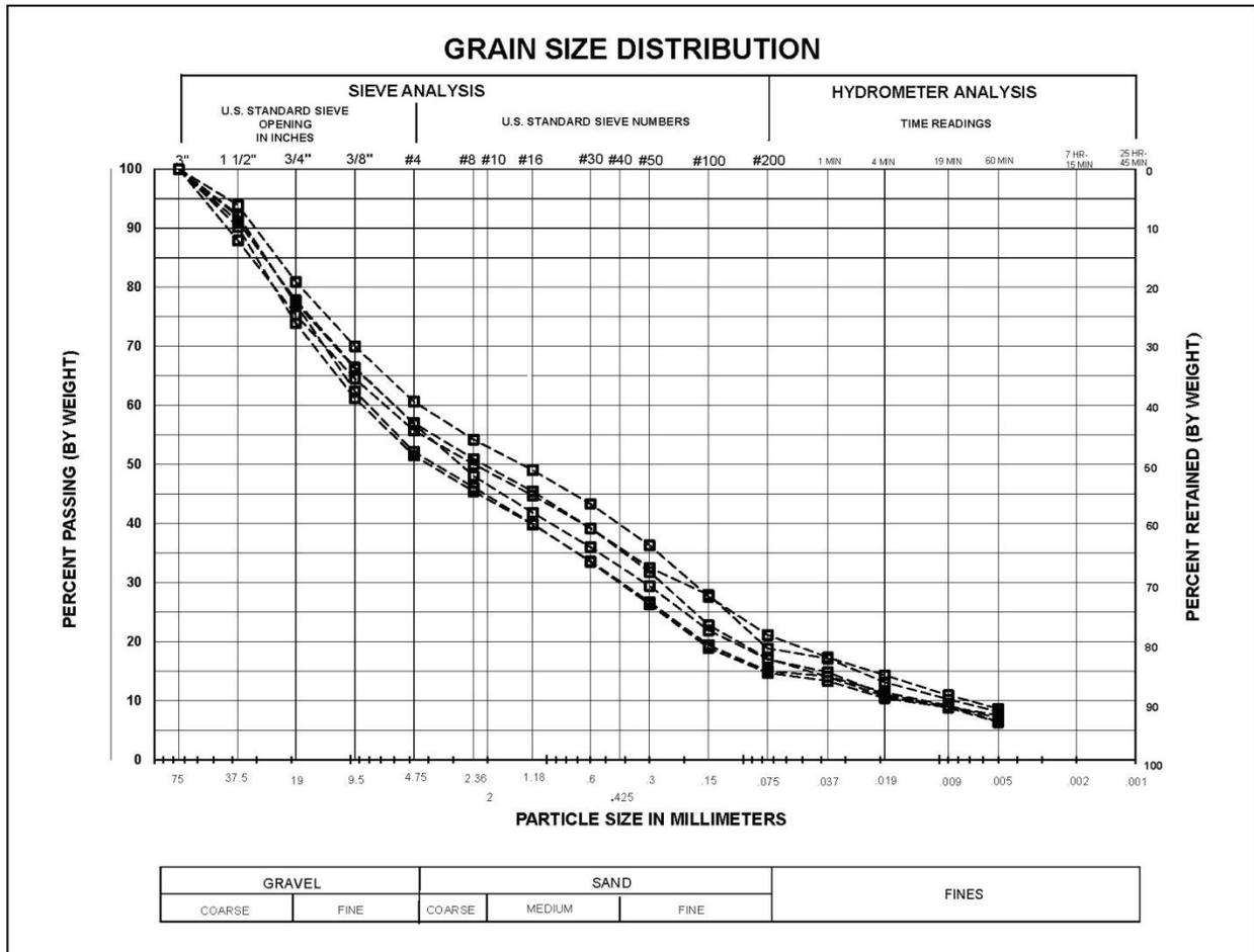
Figure 5-11. Existing embankment dam core gradations before re-grading.
