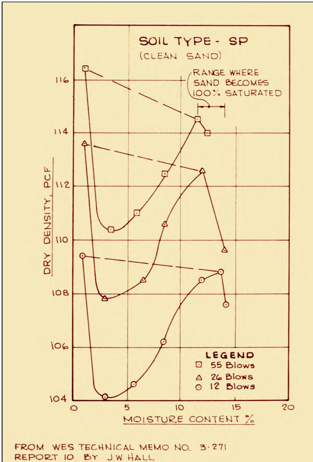
Figure 7-30. Typical compaction curves for a clean sand.
