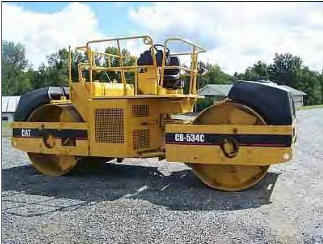
Figure 7-21. Double-drum vibratory roller.
