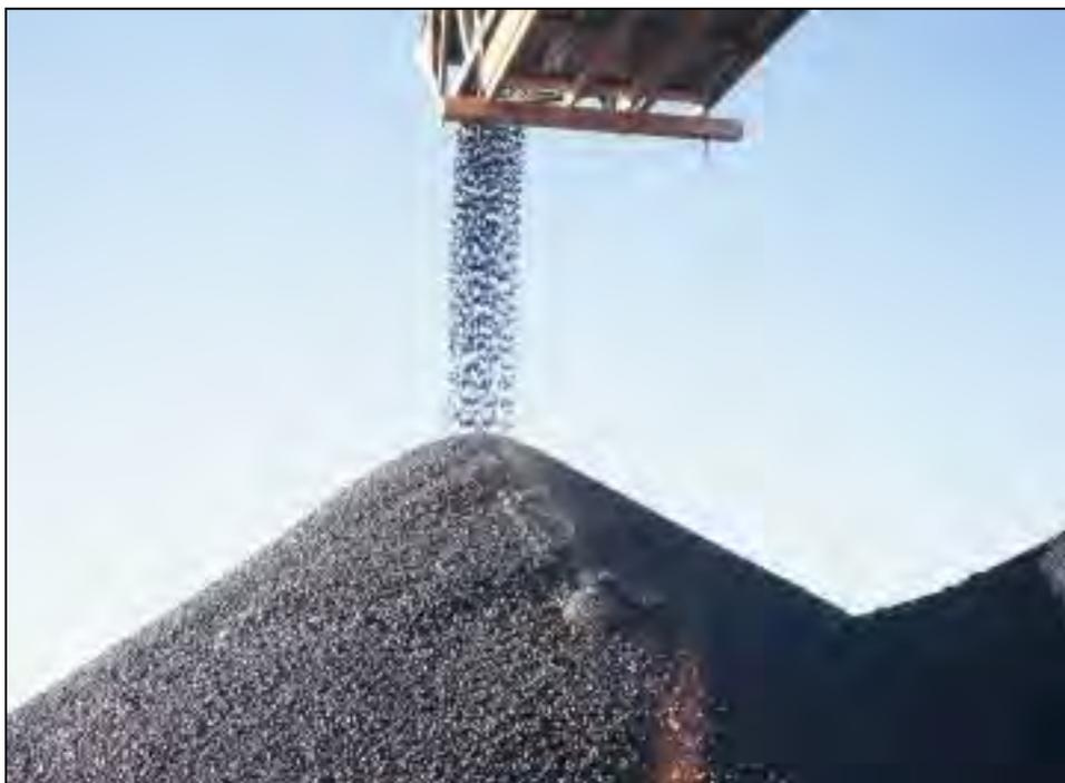
Figure 7-10. High drop height at belt discharge.
